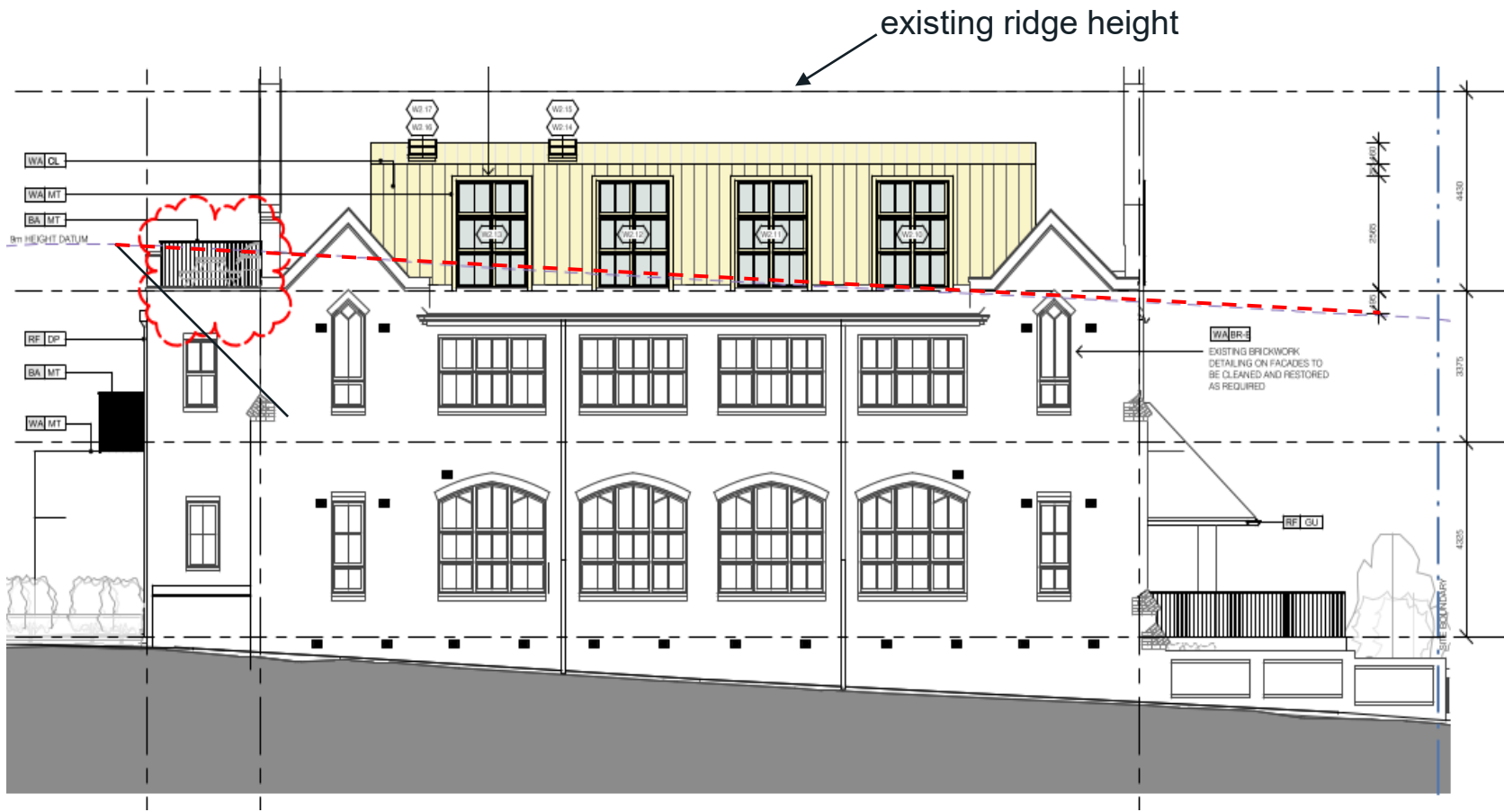
Roof additions relative to 9m height control
